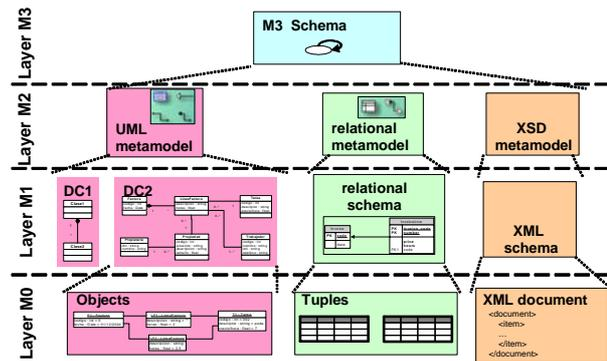
Figure 1. Graphical representation of the four-layered platform.
